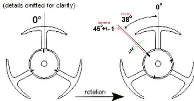
**Armature timing and the offset commutator slot relationship.**
